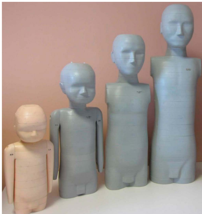
FIGURE 1. Shown from left to right are the neonate, 1-year-old, 5-year-old, and 10-year-old phantoms. Height and weight values are 51 cm and 3.5 kg for neonate, 75 cm and 10 kg for 1-year-old, 110 cm and 19 kg for 5-year-old, 140 cm and 32 kg for 10-year-old. The skeleton of each phantom is formulated with bone-equivalent materials based on the appropriate bone composition typical of each age.
