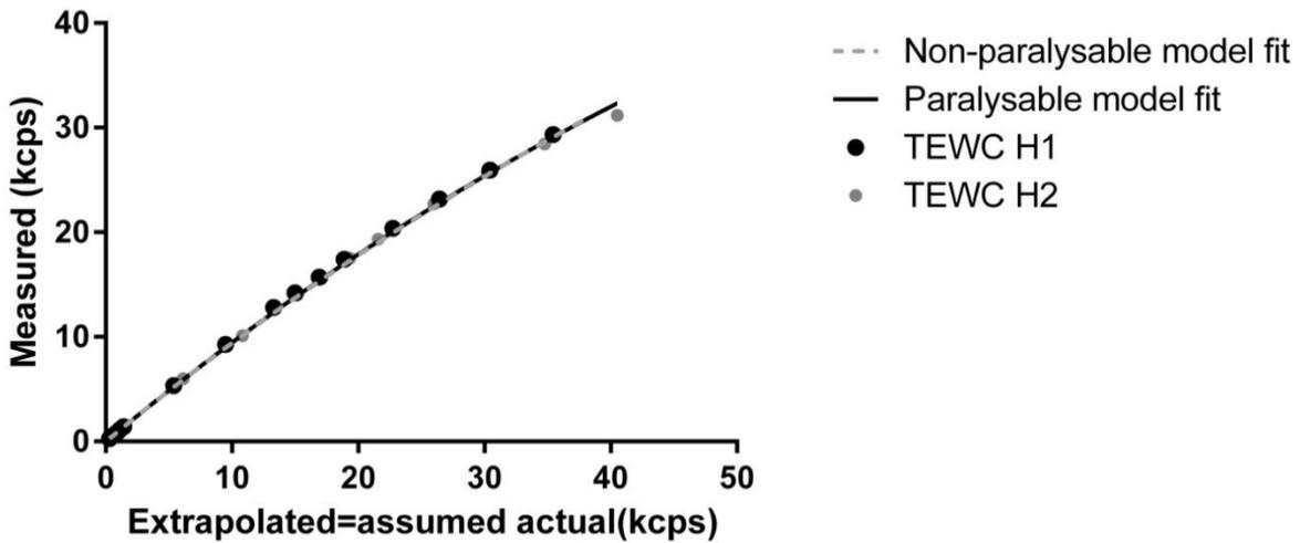
Figure 1 – measured TEWC photopeak energy window count rates a) for each head as a function of activity and b) as a function of the extrapolated count rate showing the paralysable and non-paralysable model fit.
